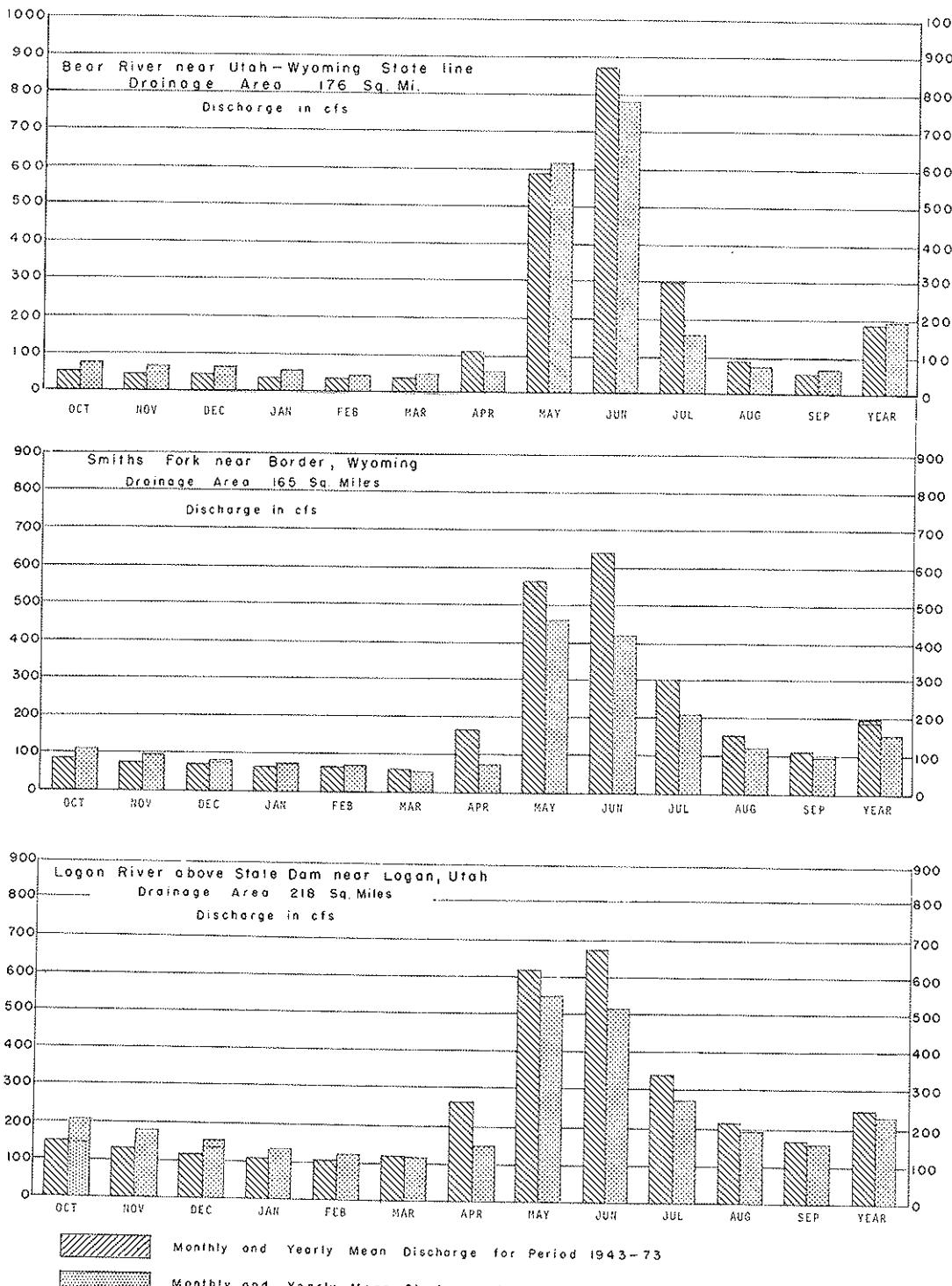
Figure 1. Comparison of discharge of three representative gaging stations in 1973 with average discharge for period 1943-73
